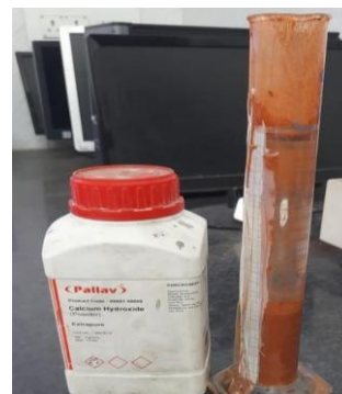
Fig. 6. Lime addition to slurry sample before settling analysis
