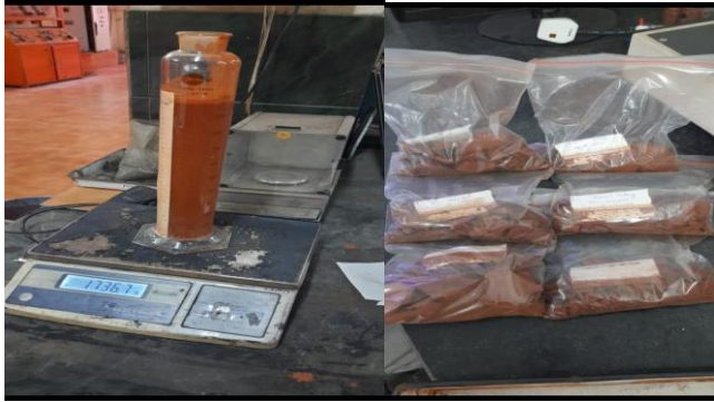
Figure 2. Weight measurement setup and dried slurry sample. Figure 3. Settling behaviour of slurry at different solid concentrations.
