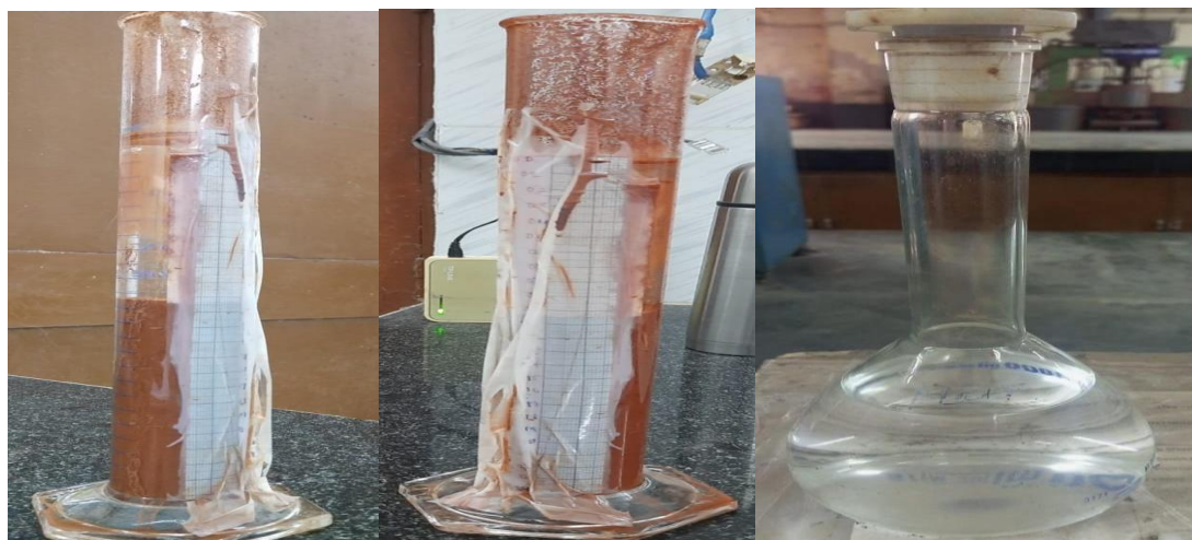
Fig. 9. Flocculant mixing and settling observation setup.
