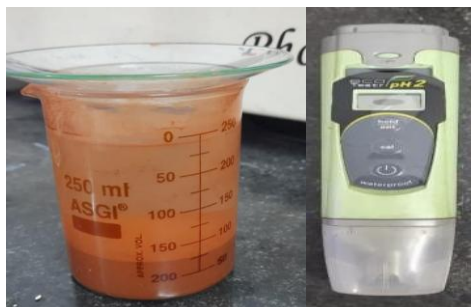
Fig. 5. Acid–base mixing setup and pH measurement arrangement.
